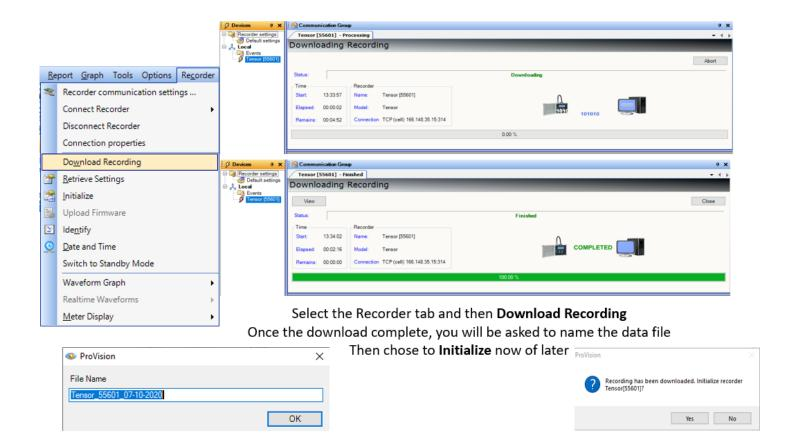
The Tensor Recorder also may be downloaded later. Simply remove the unit from the outlet and take it back to the office. The Tensor Recorder automatically stops recording when it is disconnected from an outlet. The recorded data is held in nonvolatile memory, so no data is lost.
