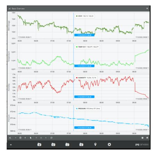
The Tensor will show Temperature, Humidity and Barometric Pressure in PQ Canvass
